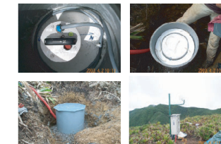
Installation of four broad-band stations. The sensors were buried in 2 meter-depth holes to avoid external noise. Azimuth corrections were computed using teleseismic Rayleigh and Love waves.
